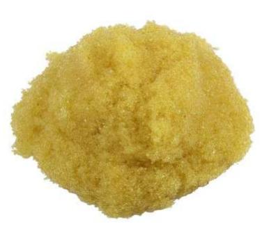
used during regeneration. PristineFlow 001x8FG can be used in water treatment systems for demineralization, for which it should be converted to the H+ form using a solution of hydrochloric or sulfuric acid.
